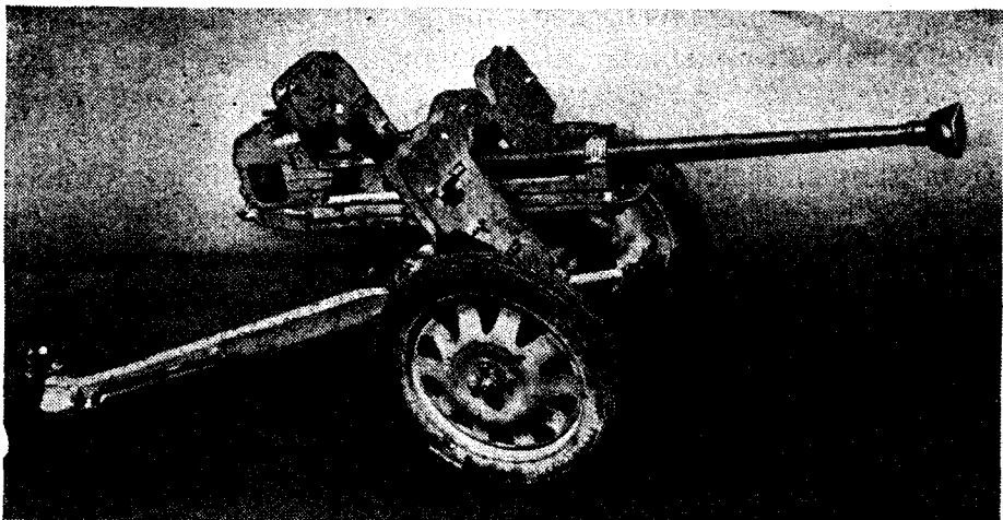
Figure 34.—28/20-mm antitank gun ( s.Pz.B. 41 ).
